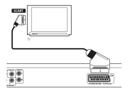
1 Use a SCART cable (not supplied) to connect the AV CONNECTOR (RGB) output to a SCART AV input on your TV (or AV receiver).
